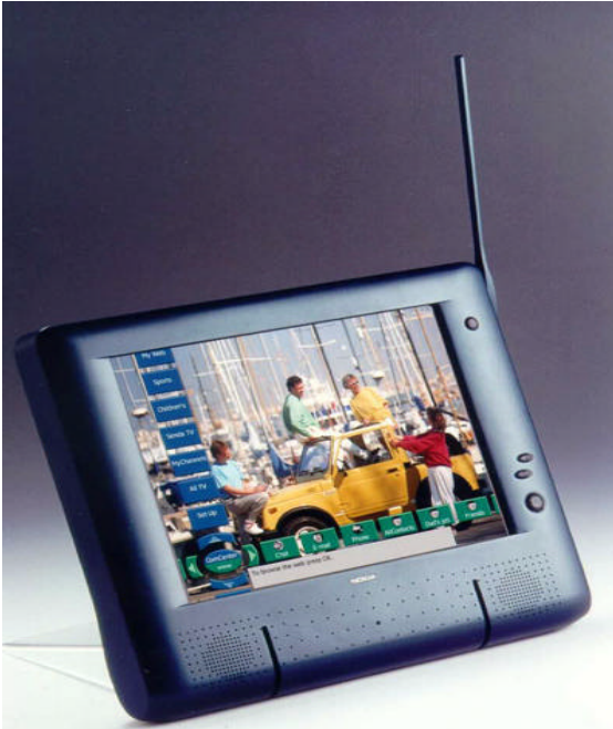
Mediamaster from Nokia (on Linux OS) combines TV, Computer, and phone into one device.
